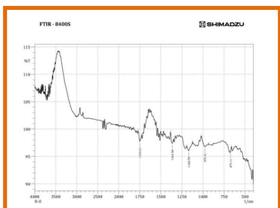
Fig3 FTIR analysis for iron nanoparticles
